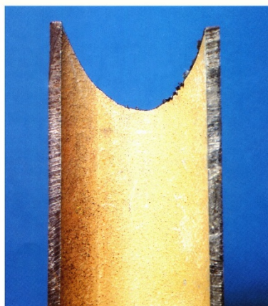
Galvanized pipe with Combiphos protective layer
