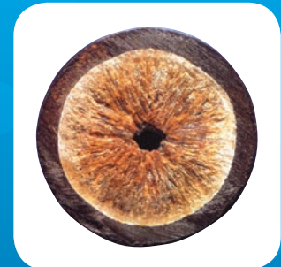
Galvanised pipe heavily scaled
