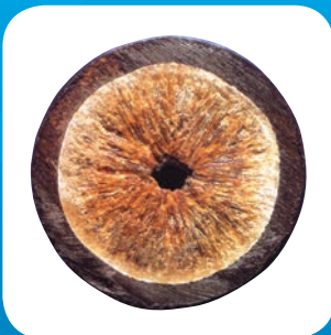
Galvanised pipe heavily scaled
