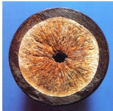
Copper pipe - heavily scaled
