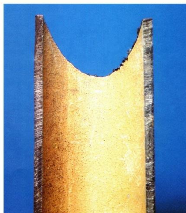
Galvanized pipe with Combiphos protective layer
