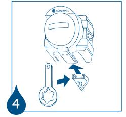
Refit red filler plug and replace front cover. Hang spanner on hook.
