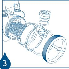
Remove dome from base, empty exhausted Combiphos and clean base. Fit new 'O' ring seal, refit dome and aluminium ring. Refill with new Combiphos through hole in dome.
