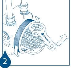
Unscrew red filler plug using the spanner provided. Unscrew and remove aluminium ring.
