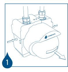
Depress the two red buttons and pull the cover away from the unit (Water flow through the unit is shut off when the cover is removed).
